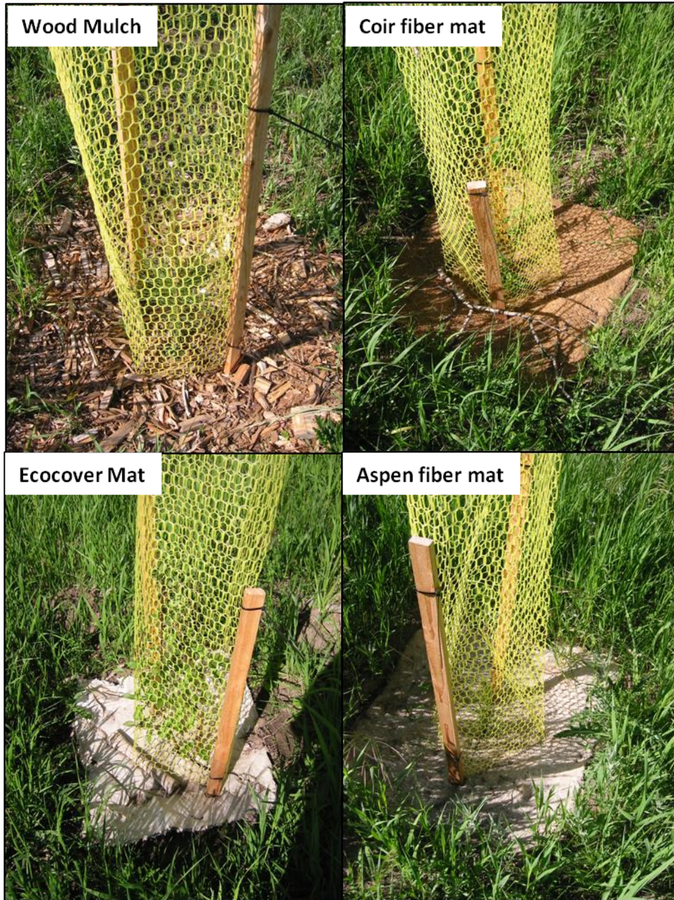
Photo 38: Biodegradable mulch products tested on Reach 2, Dry Creek. Photos were taken June 21, 2007, approximately one month after planting and installation.
